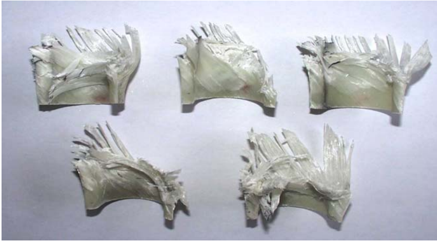
Figure 3. Energy absorption structure failure modes.
